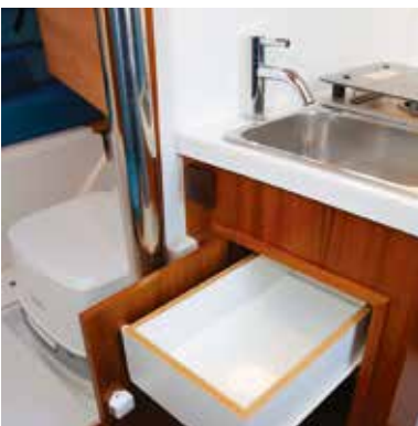
A rubber stopper protects the locker door from being damaged by the drawer
