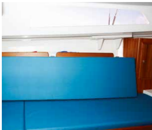
The seat backs on both sides of the saloon lift up, hinge back and clip to the hull sides to maximise berth width when sleeping
